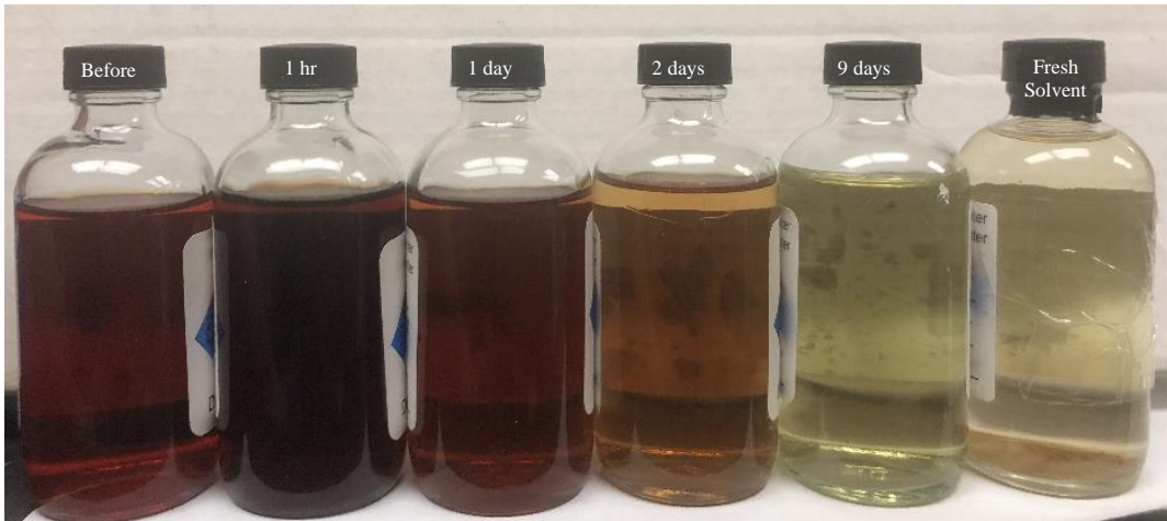
Figure 1. Solvent Color Change after the Usage of Carbon Bed
