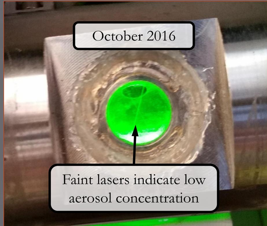
Unable to detect aerosol at water wash outlet
