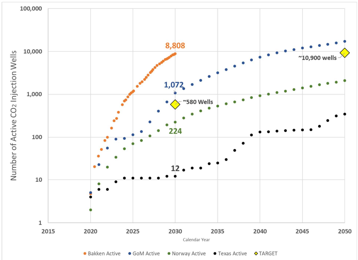
Figure 1: Projected future CO 2 injection well scenarios based on historical well development for four regions – The Bakken unconventional play in the onshore U.S. (orange; 2005-2015), the Gulf of Mexico (blue; 1947-2018), The Norwegian North Sea (green; 1966-2018), and the Texas offshore (black; 1938-2010). Target values are estimated with yellow diamond symbols, based on the IEA 2050 goal of 6-7 Gtpa and the exponential character of the curves presented.
