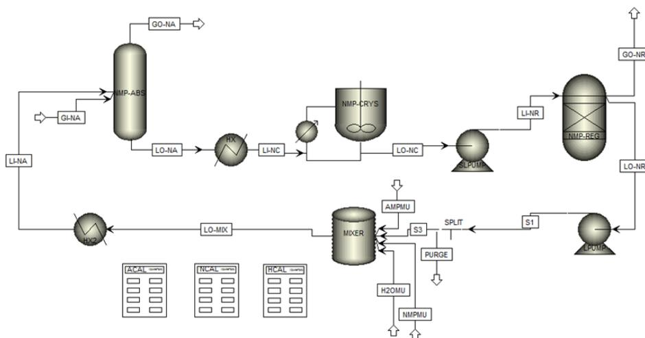
Fig. 1 The flowsheet used for modelling the AMP in NMP system
