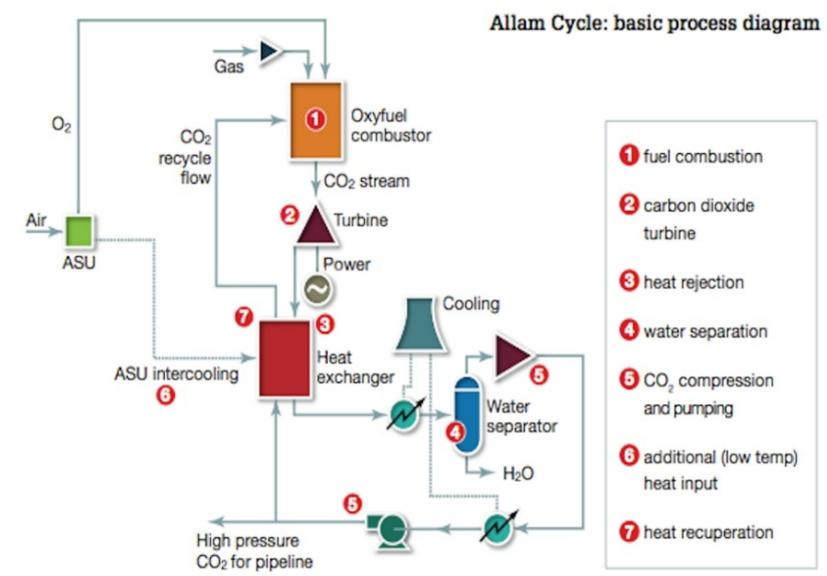
Figure 1 - Simplified Allam Cycle Schematic [4]
