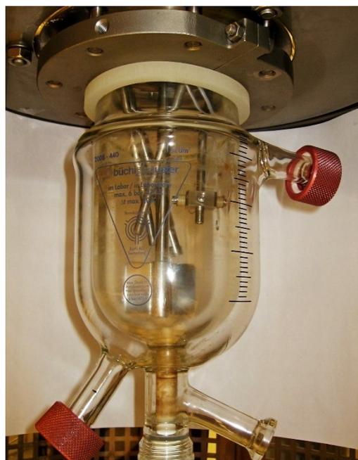
Figure 1: Büchi Ecoclave glass autoclave
