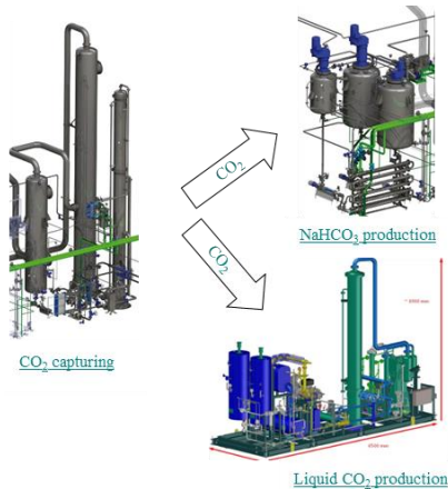
Figure 1. Schematics of Twence's CO 2 capture pilot plant
