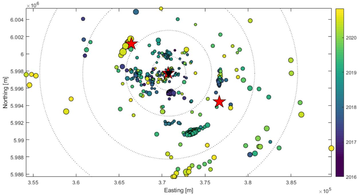
Figure 1: Map view of microseismic event locations (circles) at the Quest CCS site as of October 2020. Events are coloured by origin time. Circle size scales with event magnitude. The red stars show the three CCS injection wells. The black inverted triangle marks the location of the downhole geophone array. The black dashed circles indicate equal distances from the monitoring well ranging from 2 km to 15 km.
