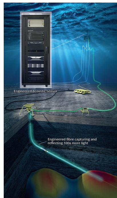
Figure 4 Long-offset subsea wells monitoring using Engineered Acoustic Sensor (EAS).
