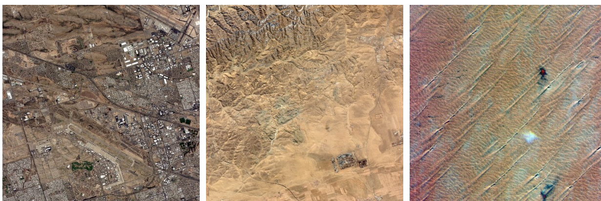
Figure 4-1: RGB images of geometric (left), spatial (centre) and radiometric (right) calibration sites captured by GEISAT Precursor.
