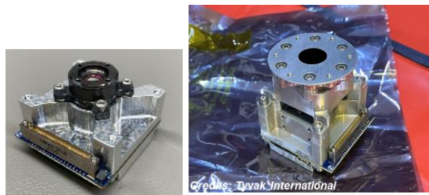
Figure 8. Milani Navigation camera (no baffle, left; with baffle, right)
