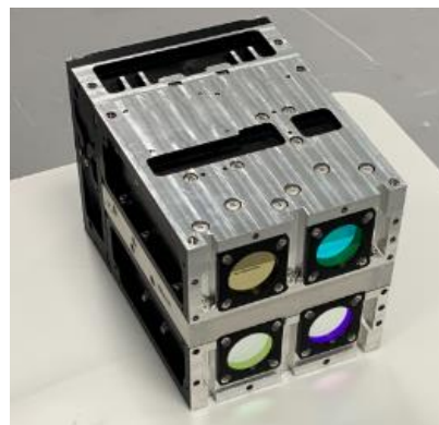
Figure 9. Milani main Payload: ASPECT hyperspectral imager
