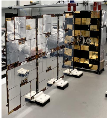
Figure 14. Milani Structural and Thermal Interface Model (STIM)
