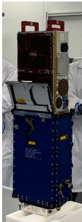
Figure 15. Milani Engineering Model and DSD fit check
