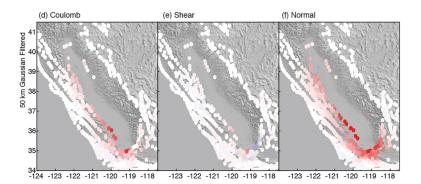
Stress field perturbation along faults in California from total groundwater loss during the 2007–2010 drought. Red color : 1-1.5 kPa stress change (Carlson et al., 2020).
