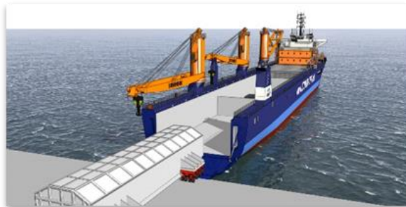
Figure 4. Loading of the Mobile Launch Box in Roll-in-Roll-Out procedure
