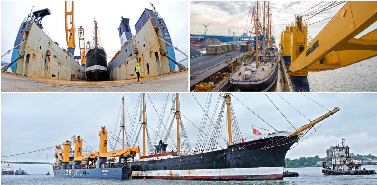
Fig. 3. Combi Dock RoRo Vessel, possible also to use as Flo Flo cargo transport (e.g. sailing ship)
