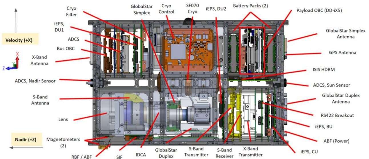
**Figure 2-2. HyTI configuration. -Y face.**
