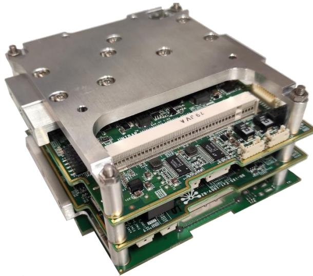
Figure 2-4. Photograph of SpaceCloud iX5-100 radiation-tolerant cloud computing solution.
