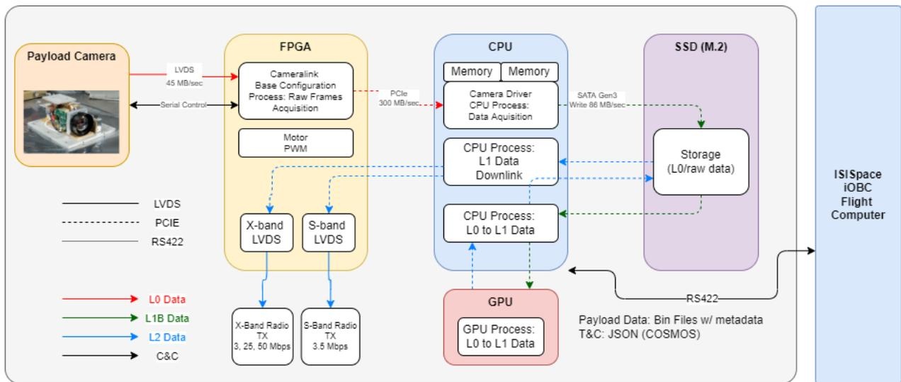
**Figure 3-1. HyTI Data Processing Flow Diagram on Unibap iX5**
