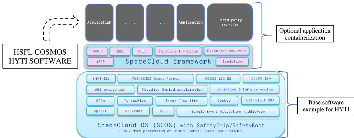
**Figure 3-1. Illustration of an expanded HYTI software stack with SpaceCloud science application containerization. HSFL COSMOS software stack illustrated in parallel to SpaceCloud Framework.**
