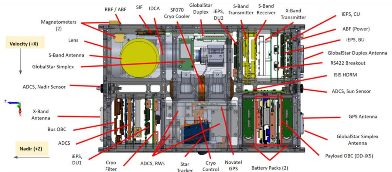
**Figure 2-3. HyTI configuration. +Y face.**
