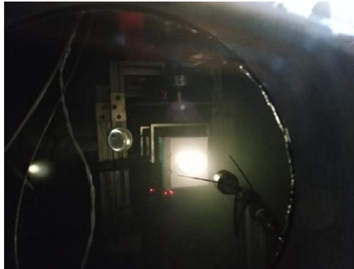
Figure 16. REGULUS B/B firing. The bright yellow colour of the plume is typical of iodine plasma.
