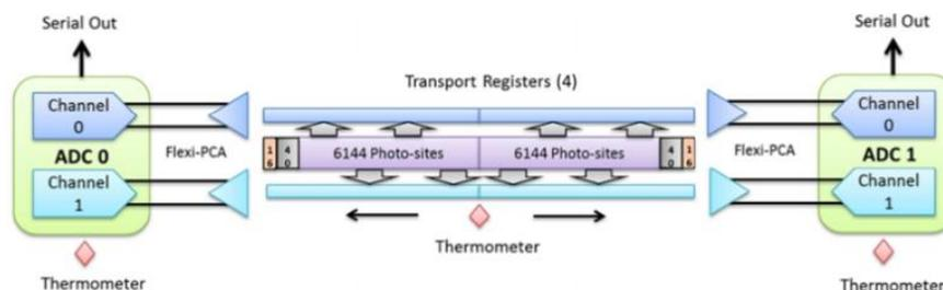
Figure 1. Single CCD 21-40. The CCD is split into two halves, with a total of 12288 light-sensitive elements. There are 40 “Dark” (covered) elements and 16 “dummy” (non-photo-sensitive) elements at each end. A total of 12496 samples will be read out per exposure (including “over-run” elements that are used in calibration). Transport registers are arranged on both sides of the photosensitive array to carry signals from “odd” and “even” elements separately.
