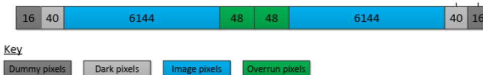
For Alsats-1B, the dark current correction is performed using the filtered Overrun pixels as follows:
