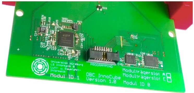
Figure 3: Redundant Skith implementation on a module board.
