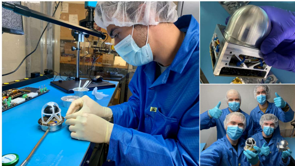
Figure 5 (Left) McMaster student, Connor Chandran, assembling and staking the vibrational support mount to guarantee the TEPC instrument's resilience during its journey to space (Top Right) The CNP-TEPC instrument, successfully built and deployed aboard the NEUDOSE CubeSat in March 2023 (Bottom Right) Photograph of the dedicated team that was responsible for designing, fabricating, and testing the CNP-TEPC instrument for the NEUDOSE mission
