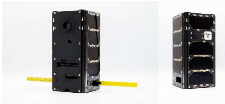
Figure 8 The flight model of the ORCASat spacecraft [A. Doknjas /CfAR]
