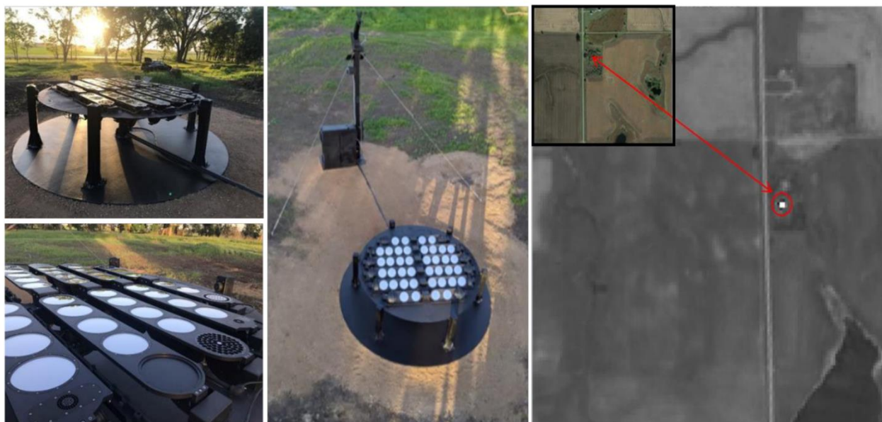
Figure 1. Beacon node installed at agricultural test site, Arlington, SD. The activated array is clearly visible in Sentinel 2B imagery (right). Inset image courtesy Google Earth. Figure reproduced from [17].
