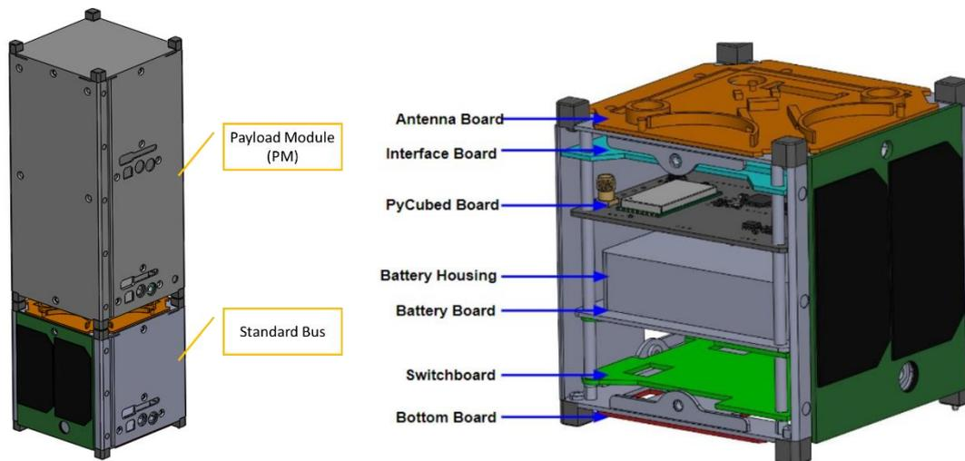
Figure 1. (Left) Notional 3U NASB-based CubeSat. (Right) Internal Layout of NASB.
