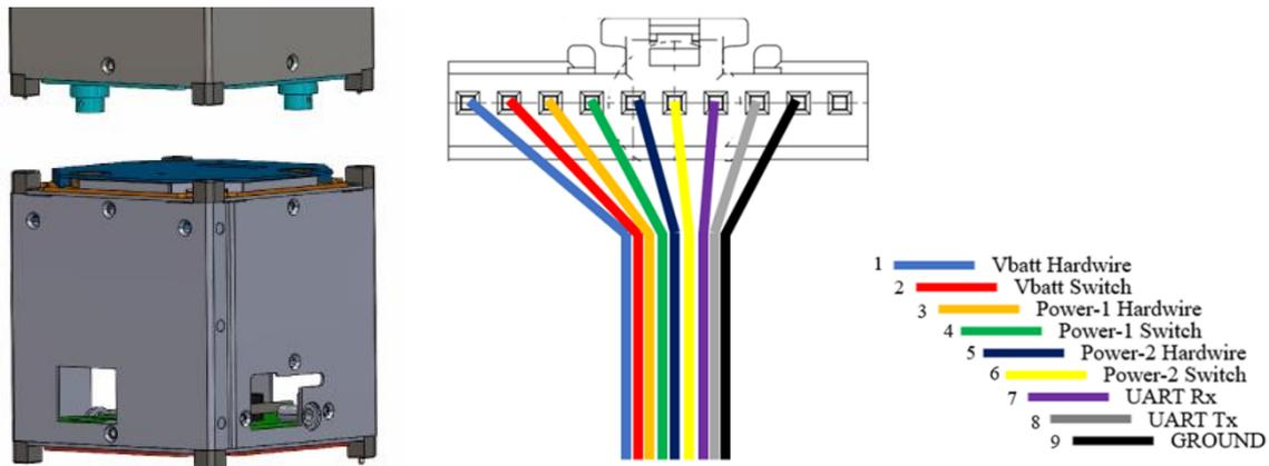
Figure 4. Depiction of mechanical (left) and electrical (right) interfaces.
