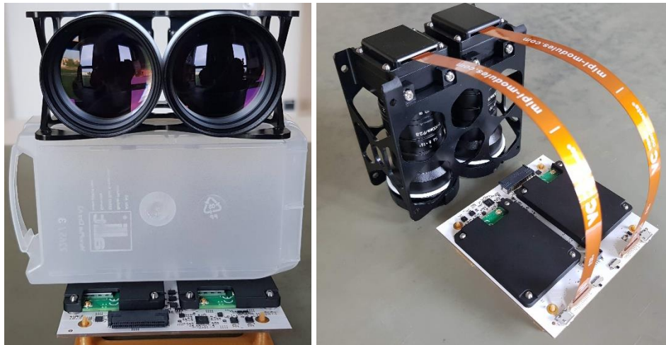
Figure 3 Redundant Camera Unit (left) and Cameras including Payload (right)
