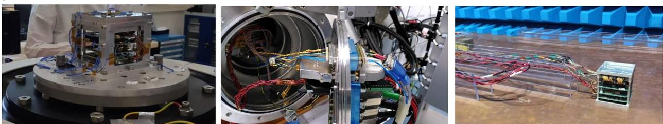
Figure 12 Environmental test setup (mechanical, thermal-vacuum), EMC
