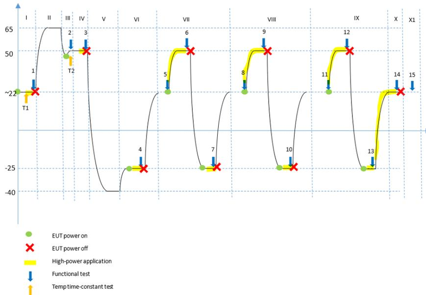
Figure 13 Thermal vacuum test profile
