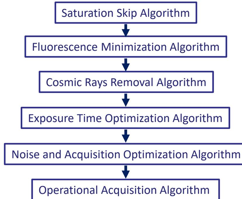
*Onboard algorithms execution flow*
