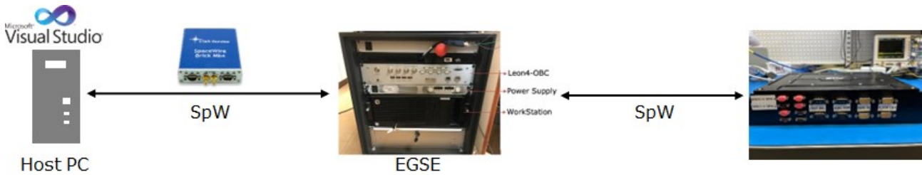
Figure 10. HW/SW codesign integration and testing setup
