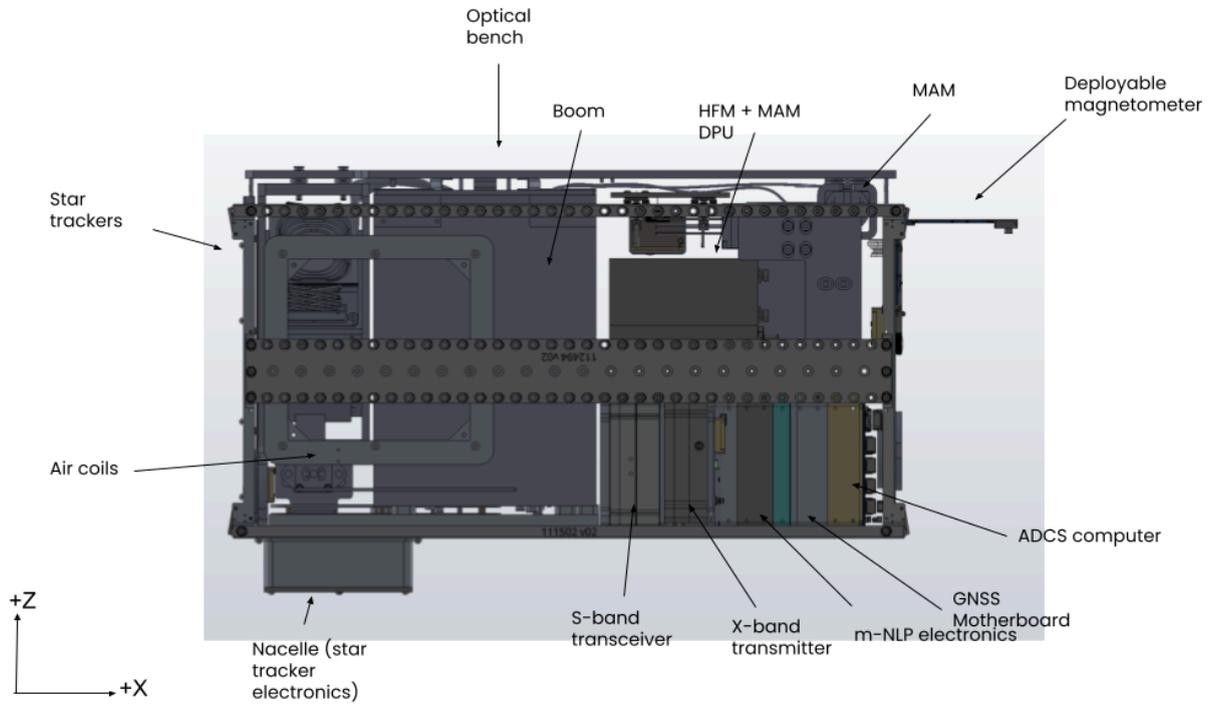
Figure 10.: NanoMagSat satellite platform design +Y view
