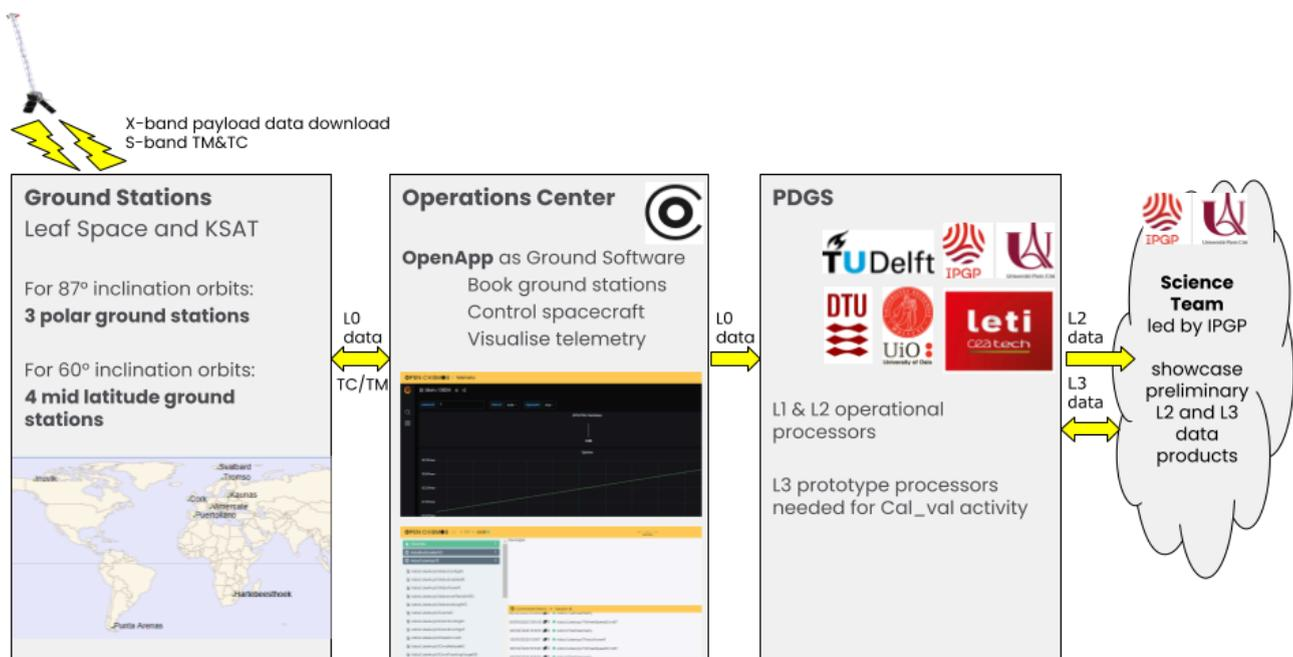
Figure 15.: NanoMagSat ground segment architecture
