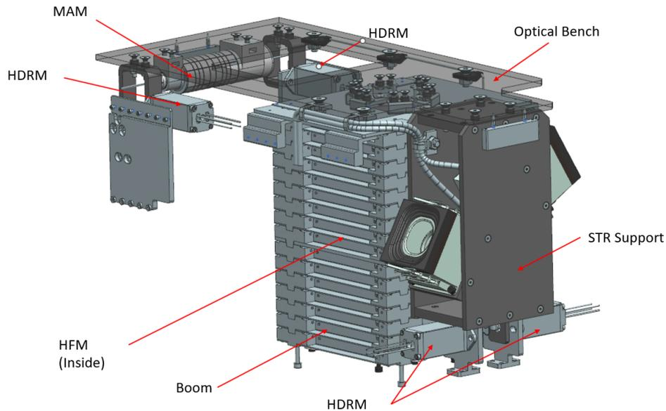
Figure 12.: payload - magnetometer suite
