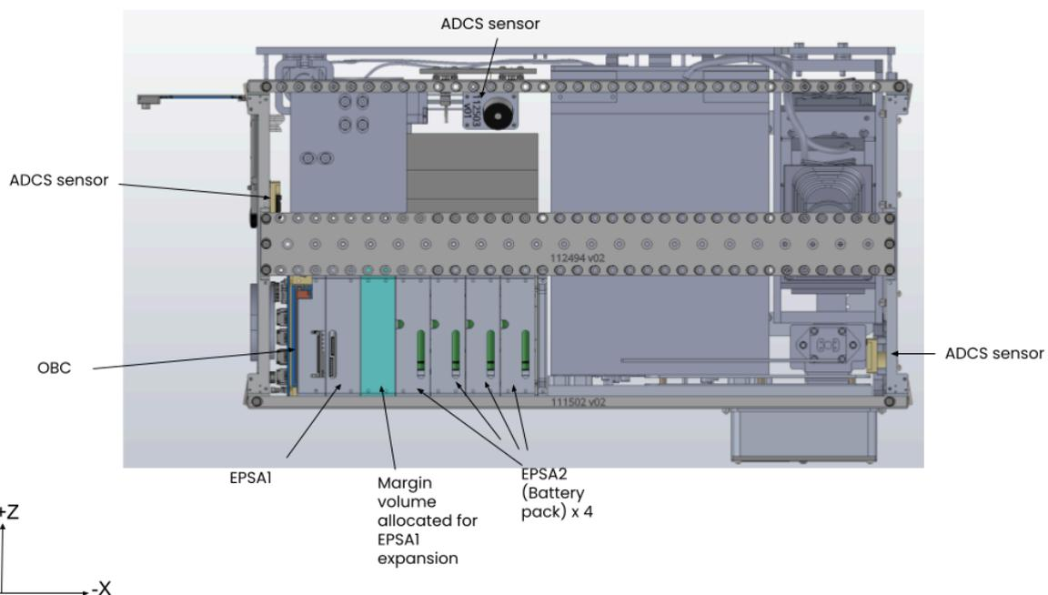
Figure 11.: NanoMagSat satellite platform design -Y view
