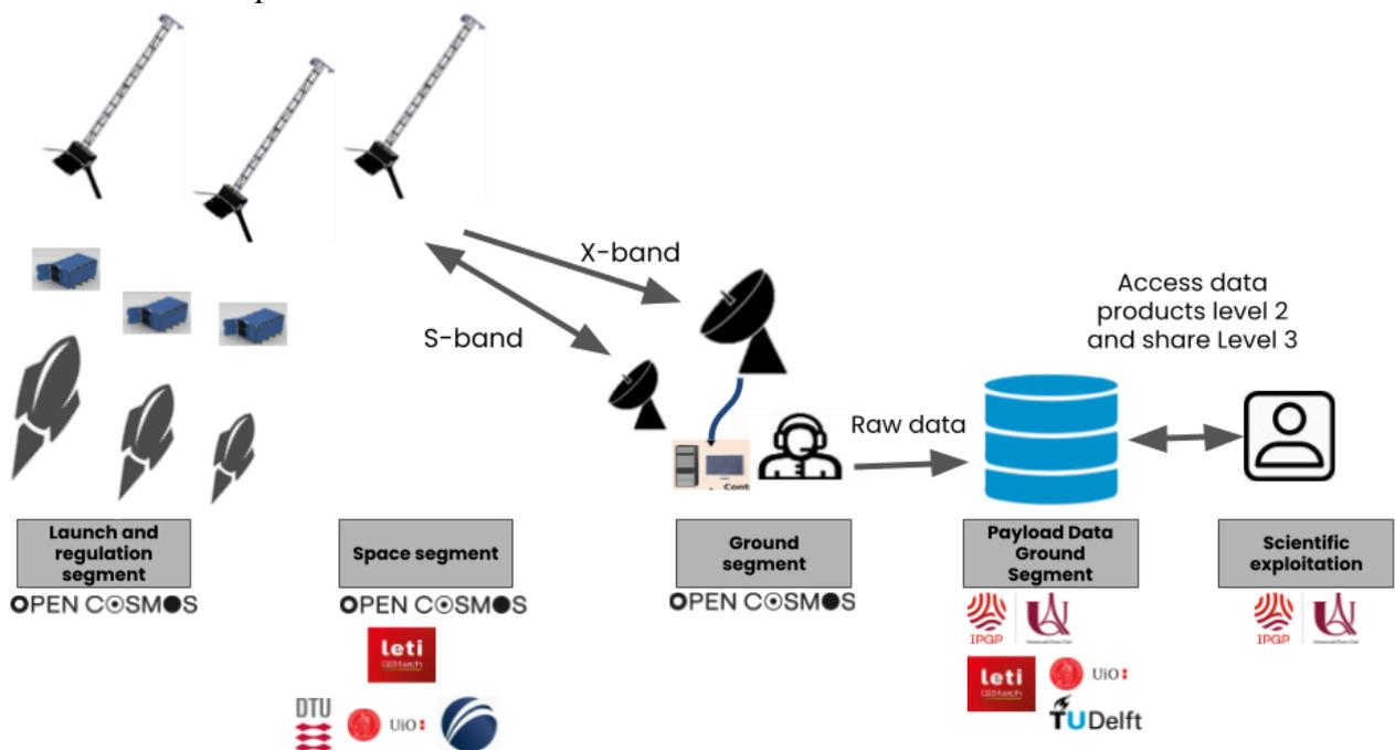
Figure 5. NanoMagSat mission architecture
