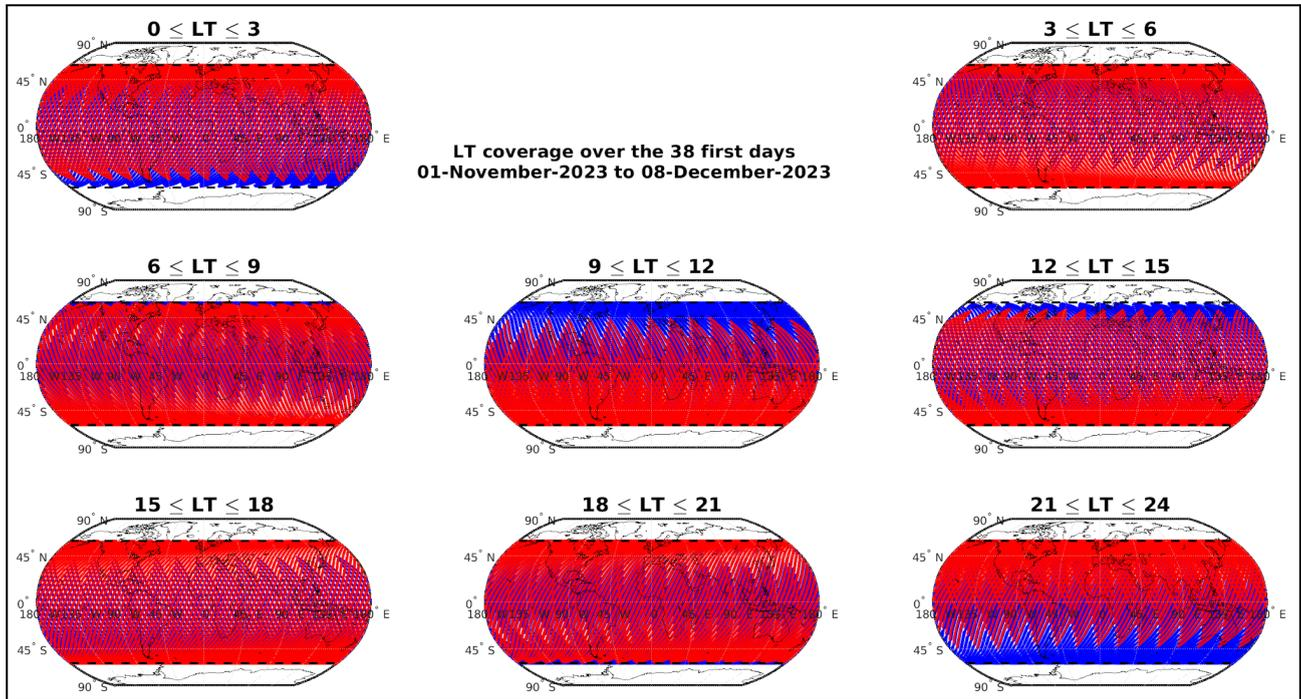
Figure 6.: spatio-temporal coverage for the  $60^\circ$  inclined satellites after the first 38 days with  $90^\circ$  RAAN separation (Note that plotting is such that red dots may hide blue dots). Credits: IPGP
