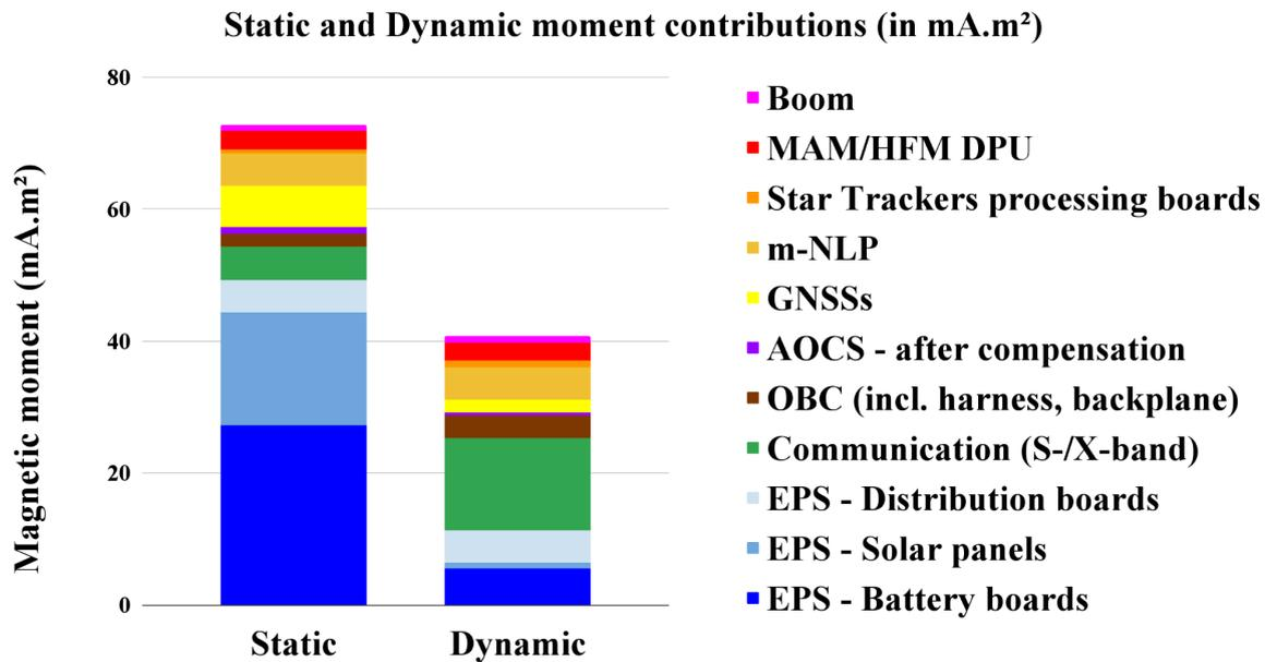
Figure 7. Static and dynamic moment contributions of the satellite based on the test carried out by CEA-Leti and Open Cosmos at CEA-Leti Herveys site in Grenoble. Note that the contribution of the tip of the boom are not included
