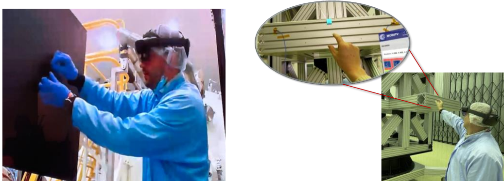
Figure 1. The VirWAIT use cases. Left: Thermocouples installation to SMILE. Right: Sensors installation to TEDY.
