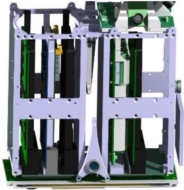
Fig. 2. Render of ICA components in the lower part of the 6U structure. Primary structure has been removed for clarity.
