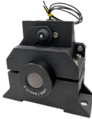
Figure 12. Photo of the ASTROtir breadboard. Within the 3D-printed housing, one can see the commercial lens in the front as well as a shutter mechanism slightly behind and above the lens.
