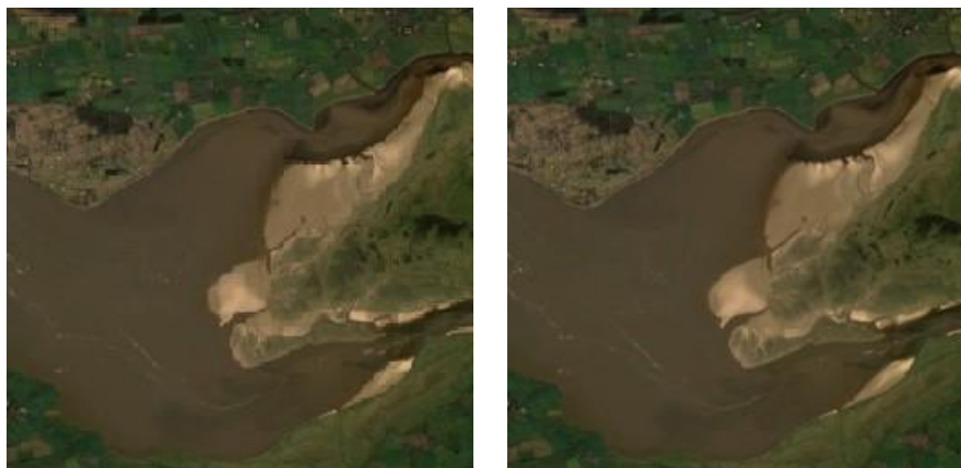
Figure 13. Landsat-9 images of Carlisle, UK, down sampled to 30m/pixel and 26m/pixel GSD respectively to demonstrate the marginal increase in resolution that would result from a decreasing altitude. Note that the image locations are normalised to enable a comparison of the GSD.
