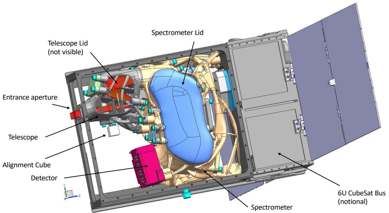
**Figure 1.** CHAPS-D instrument design, contained within a notional 6U CubeSat. The telescope (gray) and spectrometer (yellow) are additively manufactured, following topology optimization.
