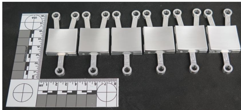
**Figure 2.** Additively manufactured CHAPS-D optical mirrors, after 3-D printing and coarse machining; before NiP plating and single-point diamond turning.
