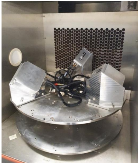
Figure 7. ARIETIS-NS EQMs in thermal chamber for performance testing
