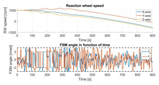
Figure 5: RW speed and FSM mirror position for scenario 1. The regions with constant FSM angles indicate FSM saturation where the it can no longer compensate the disturbances.
