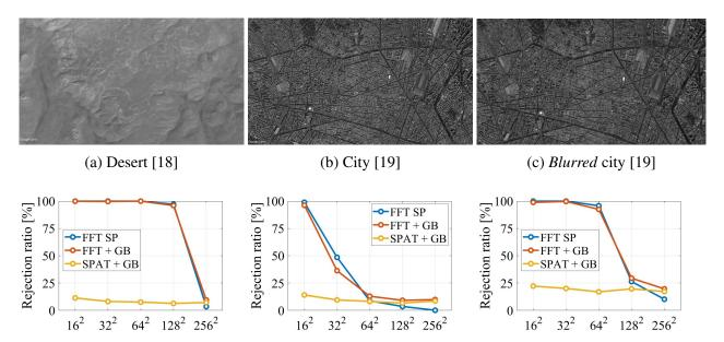
Figure 8: (Top row) Example images used for the correlation algorithm analysis. The *blurred* city image embodies a 30 pix TDI-shift. (Bottom row) The rejection ratio corresponding to the image above in function of the region of interest (ROI) size [pix<sup>2</sup>] and correlation algorithm.
