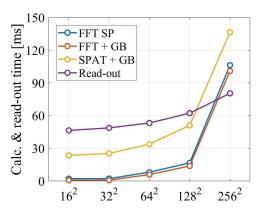
Figure 6: Calculation and read-out time in function of the size of ROI and algorithm. (Results are obtained with Python 3.8 on a HP Elitebook 840 G6 with Intel Core i7-8665U processor and 32GB RAM)
