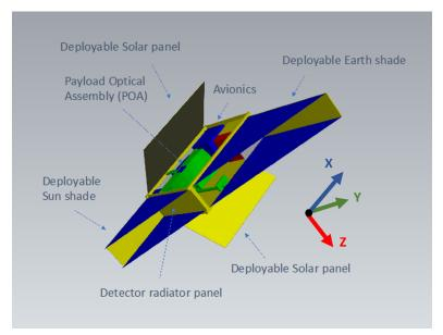
Figure 2: The CubeSpec platform with the payload, avionics and deployable panels clearly visible [9].
