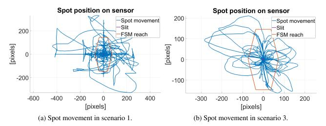
Figure 4: Spot movement during one simulation of  $15 \min$ . The red box indicates the FSM reach, the purple box indicates the slit.
