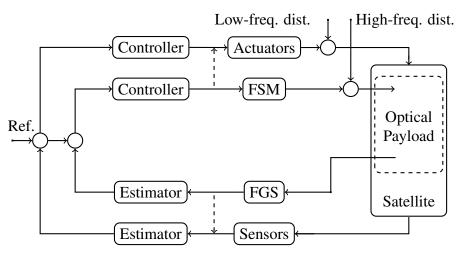
Figure 1: Control strategy of a spacecraft with both an ADCS and HPPP system. The dashed arrow below represents the potential use of FGS measurements within the ADCS estimator, as explained in section 2.4, while the dashed arrow on top represents the potential control interaction between both attitude and FSM controller, as explained in section 2.5.
