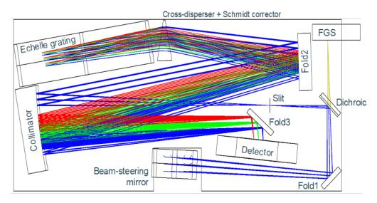
Figure 3: CubeSpec spectroscope lay-out with the science instrument and HPPP components [10].
