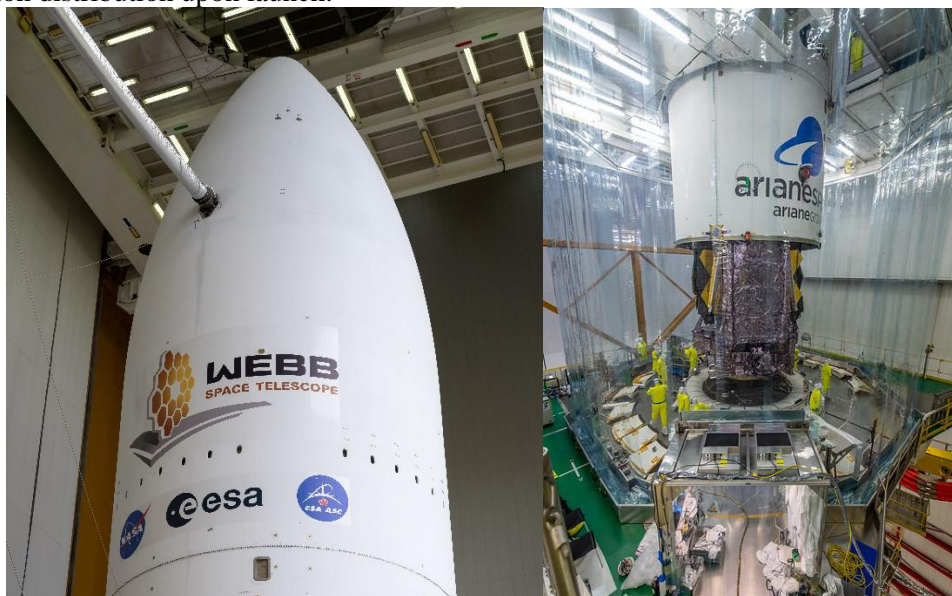
Fig. 1: Ariane 5 fairing (left) and fairing encapsulation (right) within air shower curtain (ASHC).
