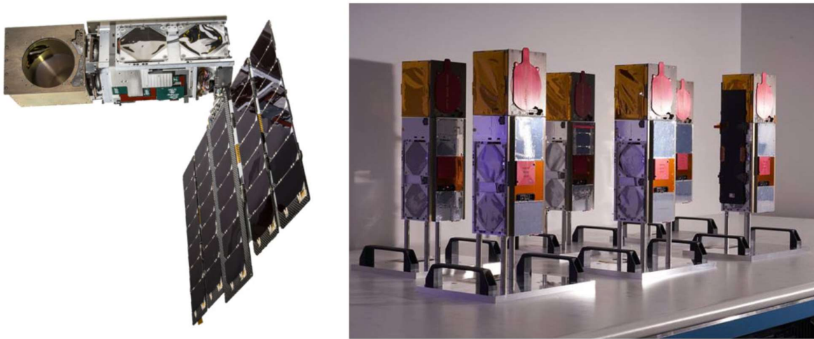
Figure 1. TROPICS Pathfinder satellite (left), showing the rotating payload connected to the satellite bus via a rotary joint. Also shown in the image on the left is the articulating solar array, which rotates (as does the satellite bus) to track the sun to maximize power output. The six satellites delivered for the constellation are shown on the right. Two of the satellites were lost in a launch failure in June 2022. (Photo credit: Blue Canyon Technologies)
