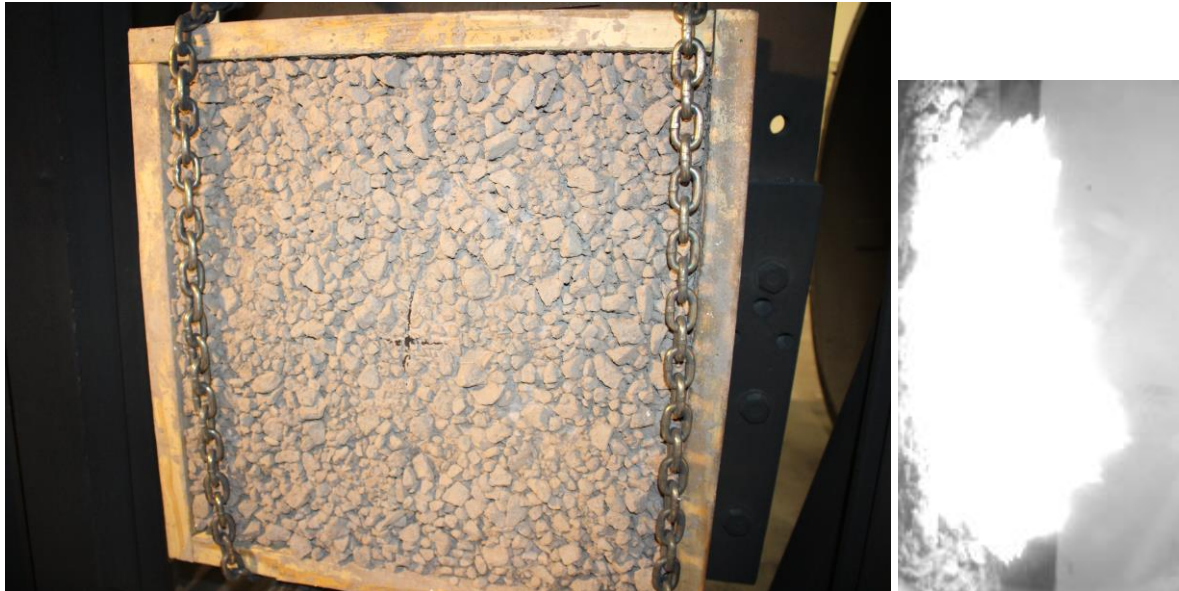
Figure 1. Left: A target hanging in the pendulum before impact showing the crushed basalt held in place by a mixture of grout and sand. Right: roughly 20 microseconds after impact (projectile came from right to left). (LGG 407)
