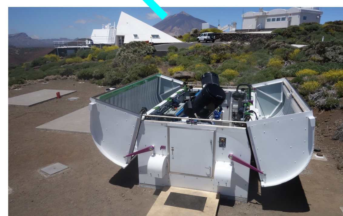
Two of LCO's 0.4-m telescopes inside their clamshell enclosure at the LCO Node on Tenerife in the Canary Islands.
