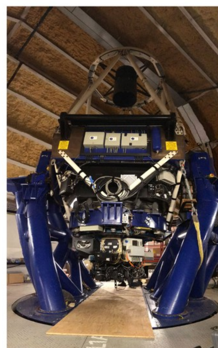
The MuSCAT3 instrument installed on the Cassegrain port of the LCO 2m Faulkes Telescope North (FTN) in Maui, HI. The FLOYDS low resolution spectrograph is installed on the same telescope on a side port and can be quickly switched to in approximately 1 minute.
