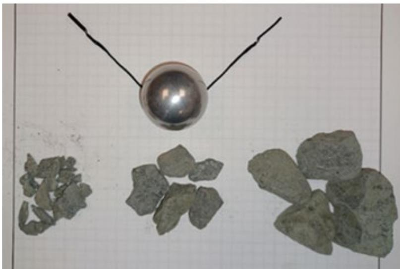
3-cm-diameter aluminum impactor and the three sizes of crushed basalt used in the study
