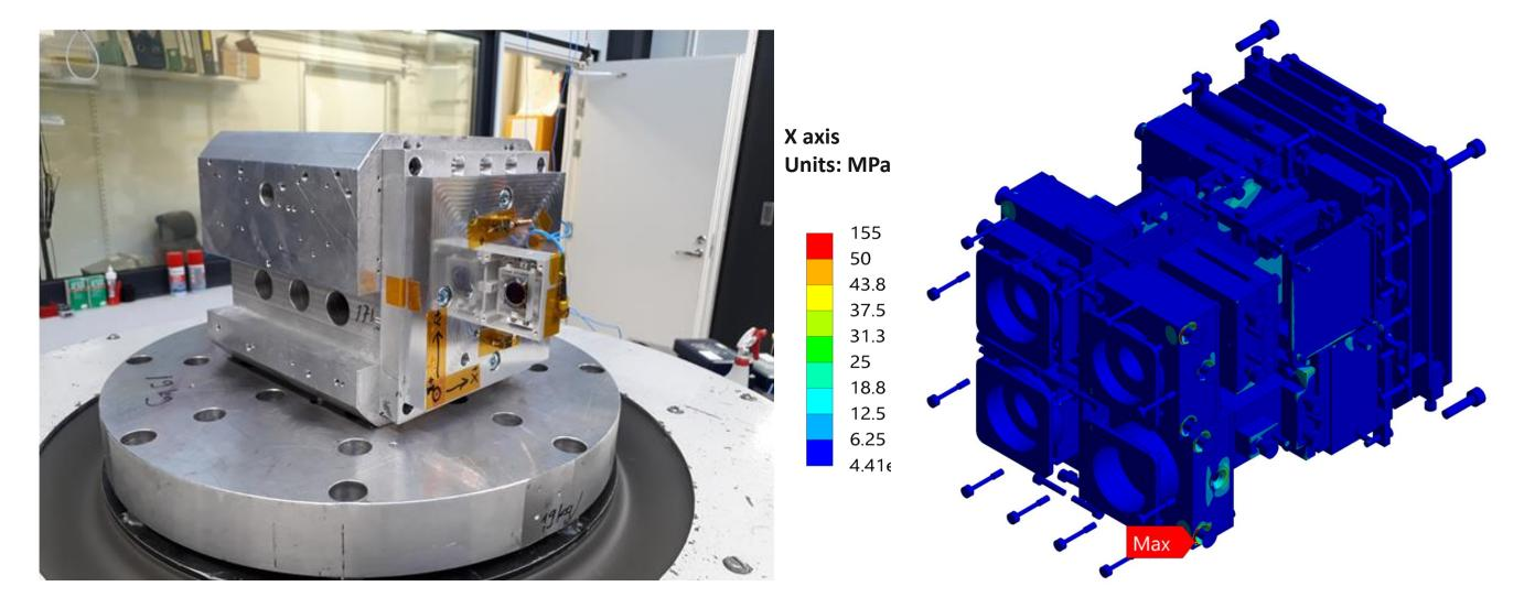
FPI vibration test assembly [Left] and Predicted Von Mises Stress for Shock Response – X axis [Right]
