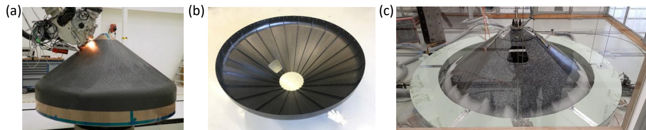
Figure 2: (a) Fibre placement of the engine frame demonstrator with steered fibre (source: NLR), (b) manufactured demonstrator and (c) Demonstrator test setup at cryogenic environment.
