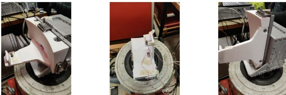
Figure 6: Macor dummy telescope undergoing shaker tests in the three main mounting configurations during launch.
