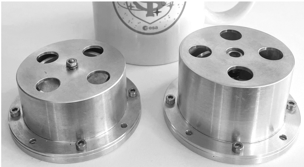
Figure 8: technology qualification prototypes: ball-bearing (left) / magnetic suspension (right)
