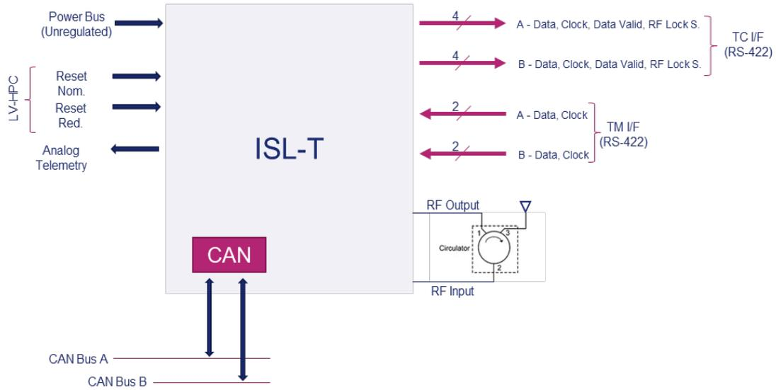
Figure 2. High-level functional block diagram of the ISL-T with the relevant external interfaces
