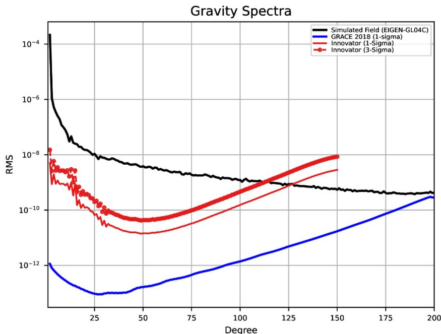
Figure 5. Comparison of the RMS of the INNOVATOR simulated estimation with the actual RMS of GRACE estimated uncertainties. The black line identifies the RMS of the Earth's gravity field model EIGEN-GL04C [11]
