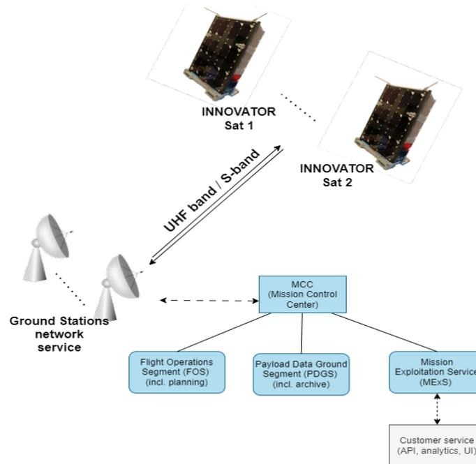
Figure 3. Ground Station System and Mission Control Centre architecture
