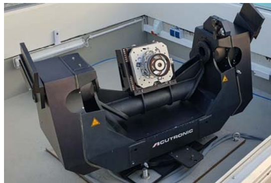
Figure 14. Jena-Optronik roof top test facility with a two-axis turntable
