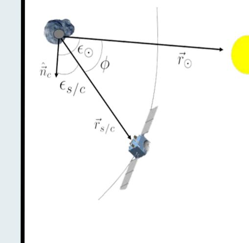
During the very-close fly-by, the spacecraft will try to image the crater at low resolutions under lighting proper conditions. Three maneuvers are used: one ground based and two autonomous.
