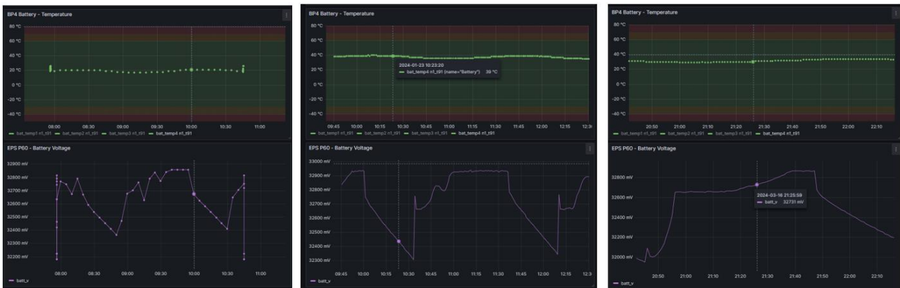
Figure 9 Battery SoC and Temperature for (left) tumbling, (centre) sun pointing, right (orbital pointing – minimum drag).
