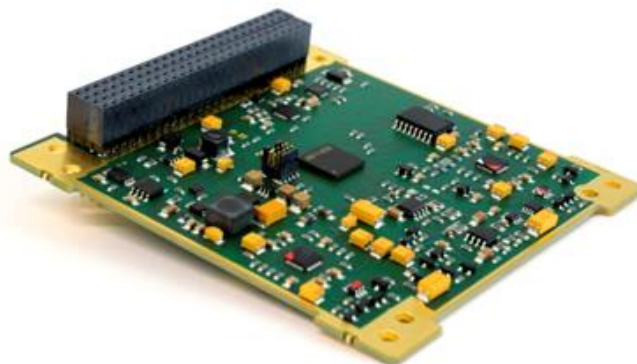
Figure 6 Photo of SATDOS, PRETTY's reference dosimeter payload.
