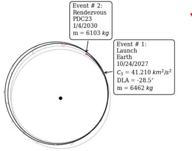
SEP is enabling for delivering the required rendezvous deflection payload without resorting to a SLS launch
