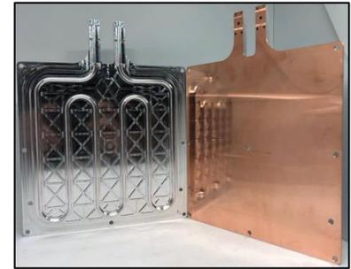
Figure 3. Left, radiator temperature as a function of power and area. Assumptions include a simplified orbiting plate and steady-state analysis. Surface properties are emissivity 0.85, and absorptivity 0.15, with a plate at 500 km altitude, edgewise tracking the sun and tilted 45 degrees viewing the earth. Right, 3D printed UAM radiators, 6U ACCS radiator (top), and 4U ATA radiator (bottom) with dual aluminum and copper layering.
