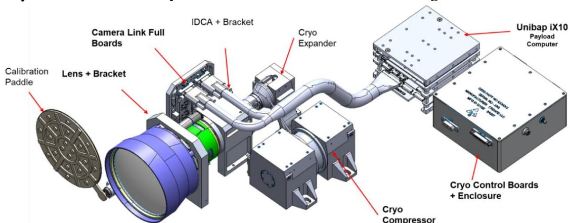
Figure 6. CAD design and component layout of the HyTI 2.0 hyperspectral instrument.
