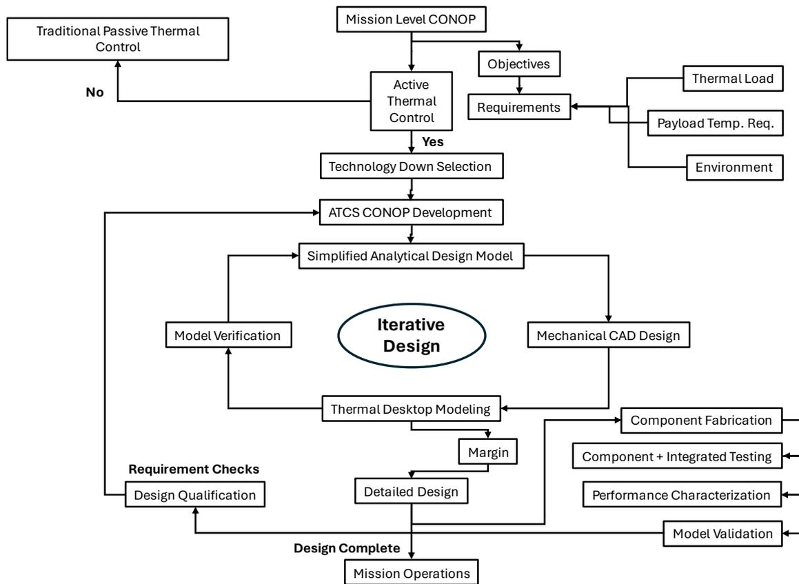
Figure 2. Space mission active thermal control design flowchart.
