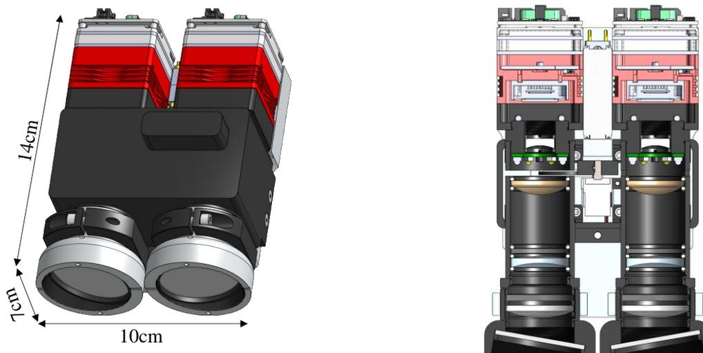
Figure 7. Left, CAD design of the FINIS instrument. Right, a cutaway view showing the camera, dual Tau detectors, and integrated calibration system.
