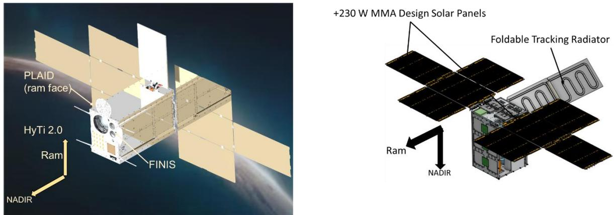
Figure 5. Left, a photo-realistic design of the 16U ACMES satellite. Right, a conceptual CAD diagram showing the high-powered MMA solar arrays and a dual folding MPFL ATA radiator.
