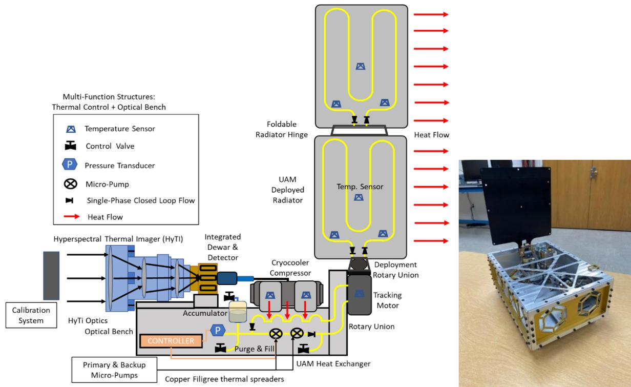
Figure 4. High-level operational concept for the Active Thermal Architecture technology. Single-phase working fluid is circulated between an internal heat exchanger and a deployed tracking radiator. The ATA system serves as the dedicated thermal control system for the HyTI 2.0 instrument, the optical bench for the telescope, and the outer wall of the spacecraft. The ATA system, 4U radiator, integrated with a 6U bus is shown on the right
