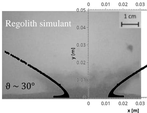
**Figure 1:** Experimental (background) and modelled (black) ejecta curtain for regolith simulant at 2.2 km/s impact velocity 0.5 ms after impact.
