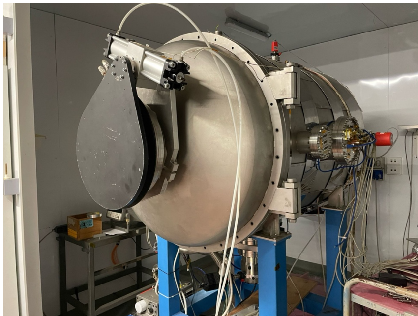
Figure 7: CISAS's thermo-vacuum chamber with window for exposition to the solar simulator.
