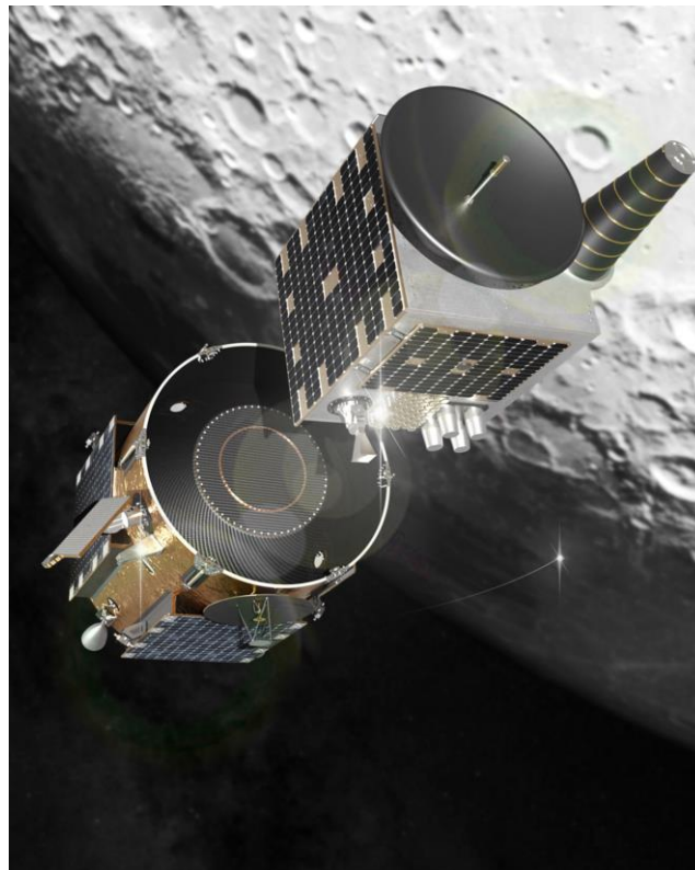
Figure 5. Blue Ghost deploying Lunar Pathfinder
